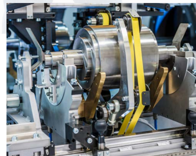
Highly precise measurement station with intelligent tangential belt drive, which folds away during measurement and therefore does not influence the measurement result.
